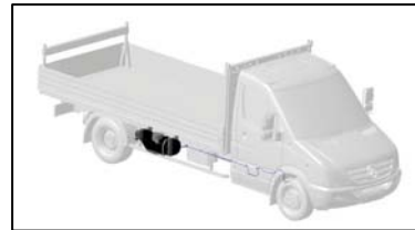
DEF Tank Location
