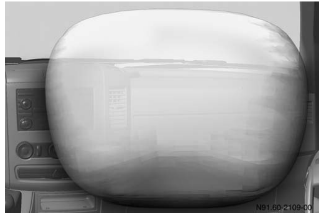
Deployment area of co-driver's airbag
