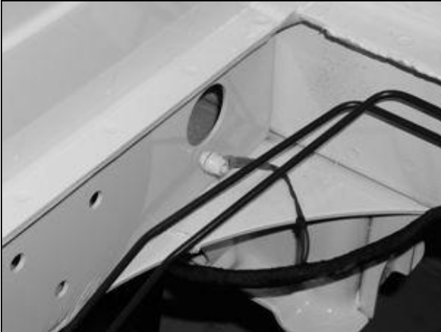
Chassis Cab Ground Terminal
