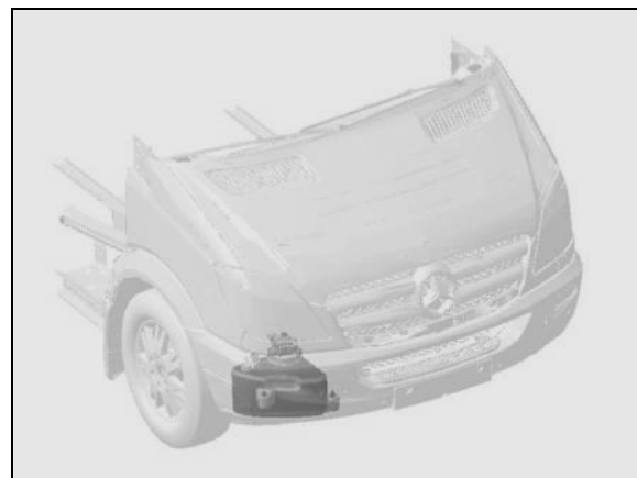
Small DEF tank location
