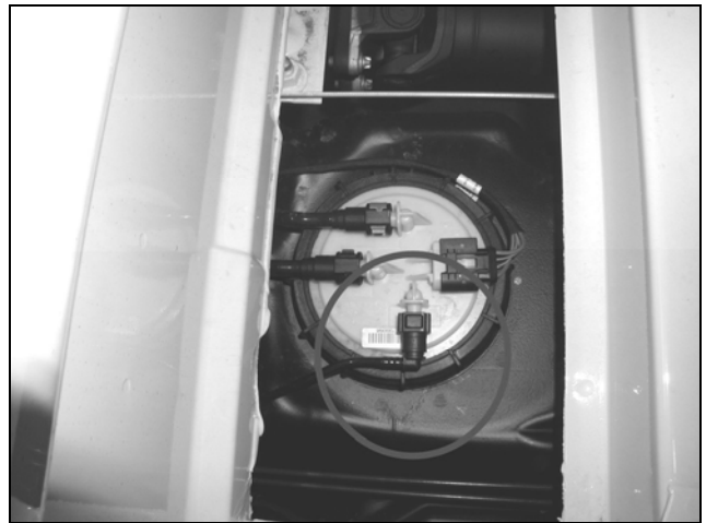
Top view showing a fuel pump unit on a chassis cab
