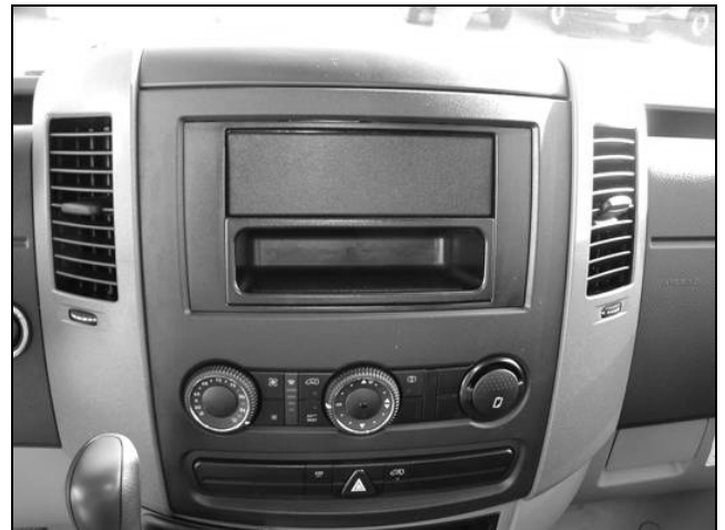
Preparation for Radio Retrofit
