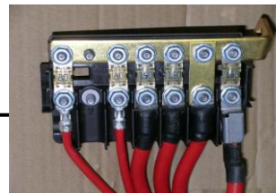
Pre-Fuse Box located on battery (+) pole
