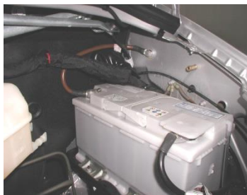
Aux Battery located in engine compartment
