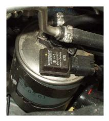
The newer Sprinters have redesigned fuel filters with the sensor located on the top of the fuel filter.
