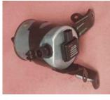
compartment down (no access that I could see from below). The connector requires squeezing across the broad part of the back end to disengage the clips. There are some similar connectors on the big hose near the radiator to give you an idea of what your fingers must look for. Here is a picture of the bottom of the filter with the bracket off to give an idea of what your fingers must find. (Don't take the bracket off. I did this because I couldn't figure out what was under the filter and how
