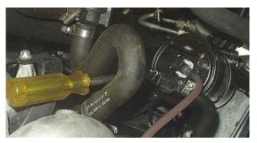
twist the fitting). This return line does double duty. In the block with the fuel return lines is a bimetal valve that directs the returned and warmed fuel<sup>1</sup> into the filter when it is cold (below 80 degrees F), or back to the tank when the filter is warm (over 80 degrees F). The picture here was taken on reassembly, so the line to the pump (step 4 above) is already in place.
