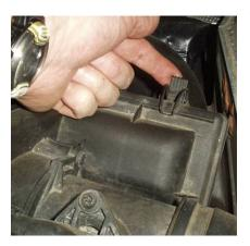
Two plastic spring tensioner tabs are located at the back of the air filter housing. Release the tabs.
