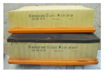
Most suppliers of Sprinter air filters offer two versions: a standard duty and a heavy duty. The two are shown at the left.
